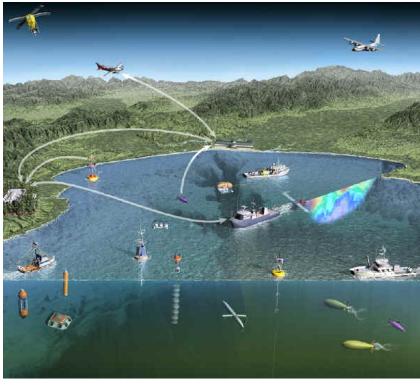
Figure 5-5: The autonomous ocean sampling network (AOSN) in Monterey Bay integrates a variety of modern platforms (e.g. satellites and AUVs) to produce a comprehensive regional view of the ocean. The network enables collaboration between different kinds of sensors. For example, an algorithm could use the network to direct autonomous submarines to explore algae blooms detected by satellites.
