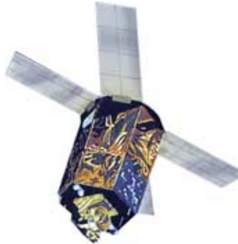
Figure 5-4: Shown above is GeoEye’s OrbView-2 “SeaStar” satellite carrying the SeaWiFS ocean color sensor.
