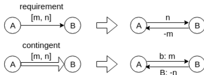
Figure 2: Conversion of temporal constraints to labeled edges in a labeled distance graph
