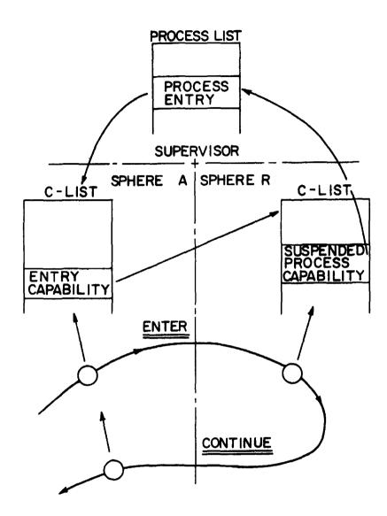
Figure 5. Entry to and Exit from a Protected Procedure
