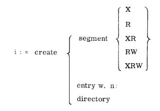
A capability pointing to the created object is entered into the C-list of the process with an O indicator, and its index number is reported as i. Note that a name is not associated with the object at the time of its creation, but only when an entry is made for it in some directory by means of a place meta-instruction.
