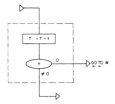
Figure 2. The join Procedure Step
