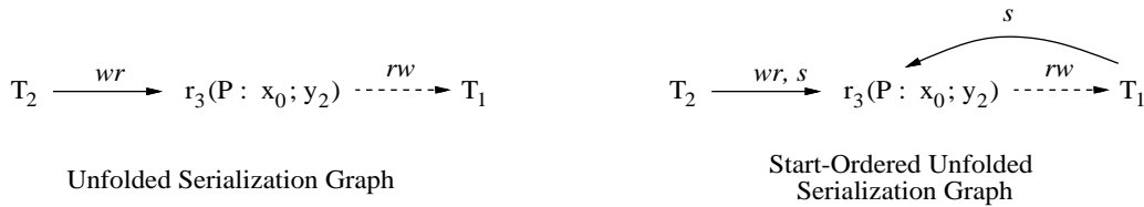
Figure 4-11: History H_{non-MSR} is accepted by isolation level PL-2L but not by PL-MSR.
