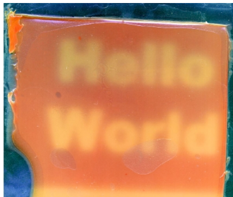
Figure 2d. Students at UT Austin used the image 'Hello World' to illuminate a ~10cm square lawn of bacteria containing their initial system (the first picture encoded on their biofilm film is shown here). A lawn of E. coli should be able to capture images at about gigapixel per square inch resolution. Photo: Jeff Tabor.
