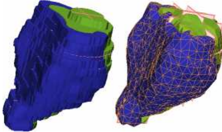
Figure 2-1: Left: Surface of voxel representation of a prostate central (green) and peripheral zone (blue). The region encompasses eighty thousand voxels. Right: the same region represented after smoothing the left surface and filling with tetrahedra. The brown lines represent the surface edges of the mesh. The region is described by seven thousand tetrahedra. The tetrahedra-based representation is much smaller than the voxel-based representation and better describes the expected smooth surface of the prostate.
