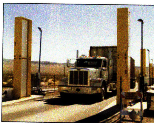
Figure 7. Advanced Spectroscopic Portal (ASP) (Source: Defense Dept. Doubles Spending on Systems that Don't Deliver, from http://www.cnet.com/military-tech/?keyword=GAO ed )
