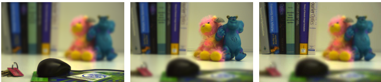
Figure 16: Synthetic refocusing using the coarse depth map estimated with the lattice-focal lens.
