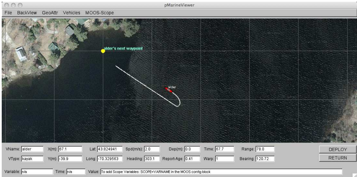
Figure 10: The SimpleWaypoint behavior in action: After the vehicle has reached the waypoint prescribed in the transiting instance of the SimpleWaypoint behavior, the second instance of the SimpleWaypoint behavior, returning to the start point, becomes active.
