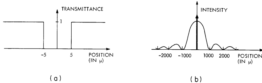
Fig. XI-19. (a) Input transmittance of a simple spot. (b) Expected output image for the input of (a).
