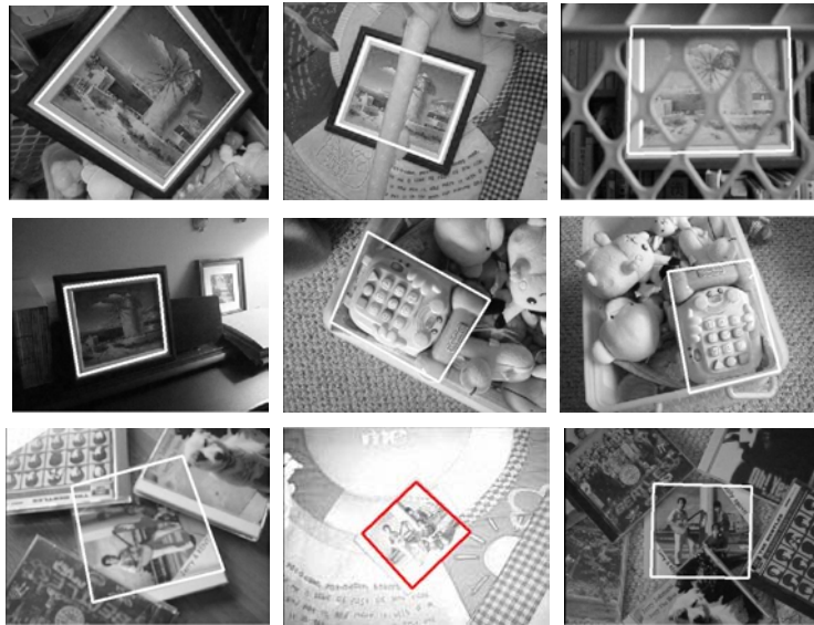
Figure 12. Objects are detected under different environment in different pose. 320x240 images taken under various environments with changes in illumination, scales, rotations and perspectives. Even a CD taken with flash and a painting with occlusion are robustly detected.
