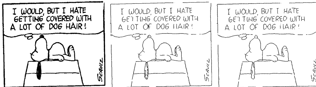
Figure A-3: Elimination of small “bubbles” in the thinned image using the method described in the text. On the left, the original binary image. In the middle, the image after morphological edge extraction, but with bubbles. On the right, the image after removal of small bubbles using the method described in the text.
